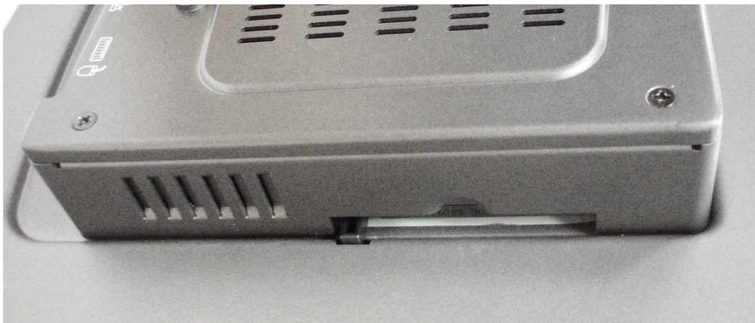
**Figure 2.2 Install CFast Memory Card**
